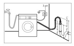
The drain hose may be extended to a maximum of 4 metres. An additional drain hose and joining piece is available from your local Service Force Centre. The joining piece must have an internal diameter of 18 mm. If your drain hose looks like this (see below) you do not require the "U" piece". Just push the hose firmly in to the standpipe.
